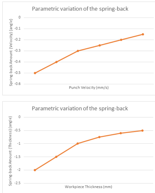
Fig. 5. Parametric variation of the spring-back amount: (a) to the punch velocity; (b) to the workpiece thickness
